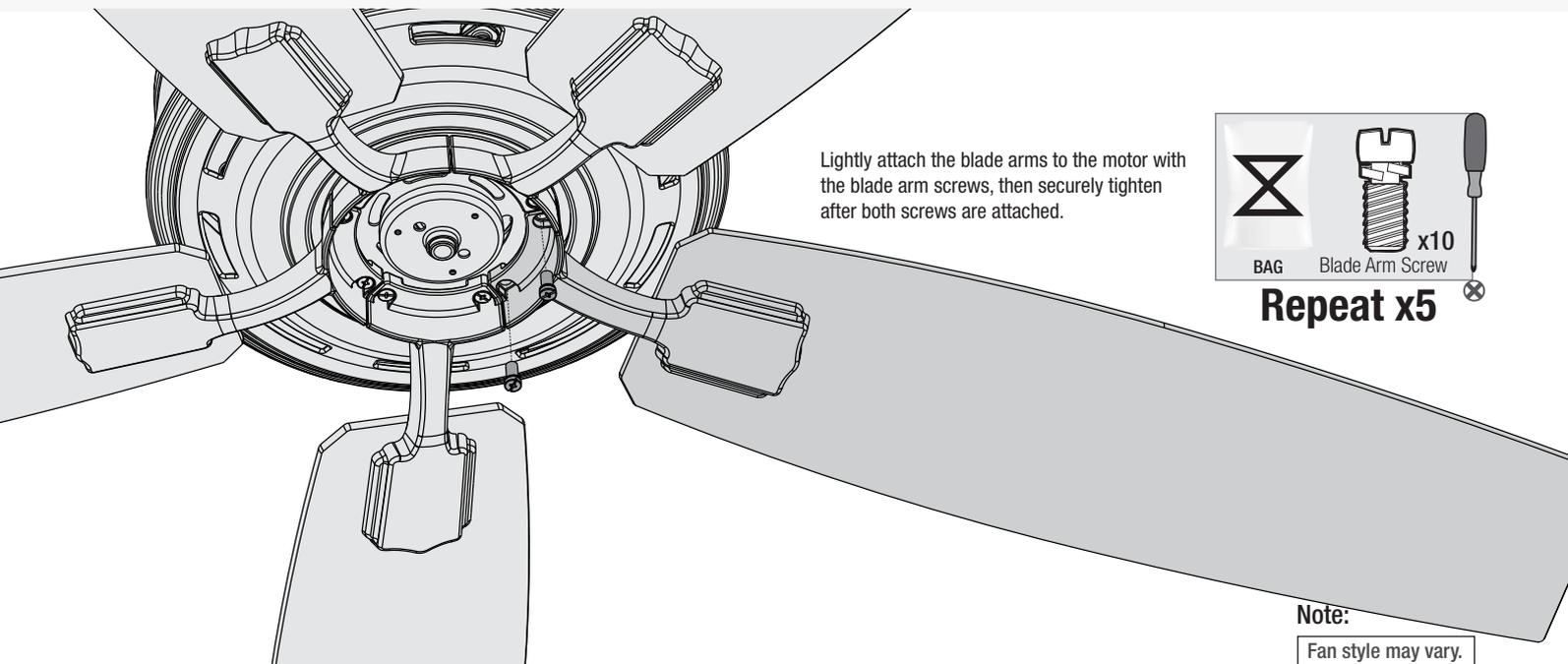
Lightly attach the blade arms to the motor with the blade arm screws, then securely tighten after both screws are attached.
