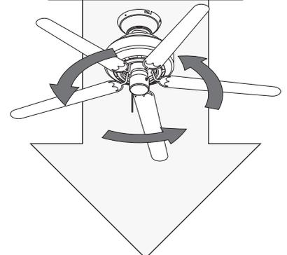
Downdraft (counterclockwise rotation) creates a direct breeze and maximum cooling effect.
