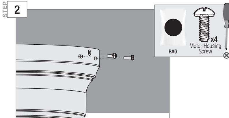
With a Phillips head screwdriver, install the four motor housing screws found in the hardware bag. Tighten all four screws securely.
