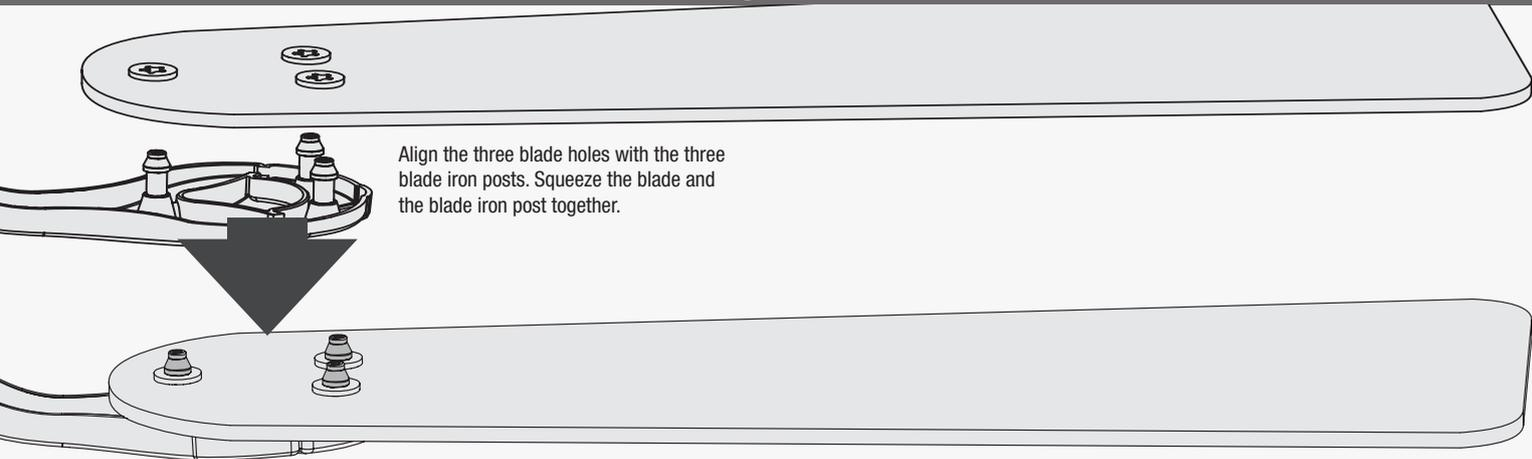
Align the three blade holes with the three blade iron posts. Squeeze the blade and the blade iron post together.
