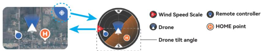
The attitude indicator displays information of drone direction, tilt angle, remote controller direction, HOME point and more.
