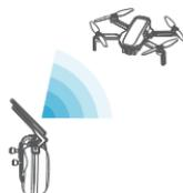
When the drone is directly above the remote controller, the transmission signal is significantly weakened due to the poor antenna angle. To address this, please lower the flight altitude or fly the drone horizontally for some distance, ensuring that the antenna points towards the drone as much as possible, as shown in the picture.
