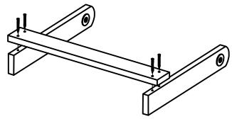
**3)** Attach Back Support Brace (shorter piece) to Back Support Sides with four A screws.
