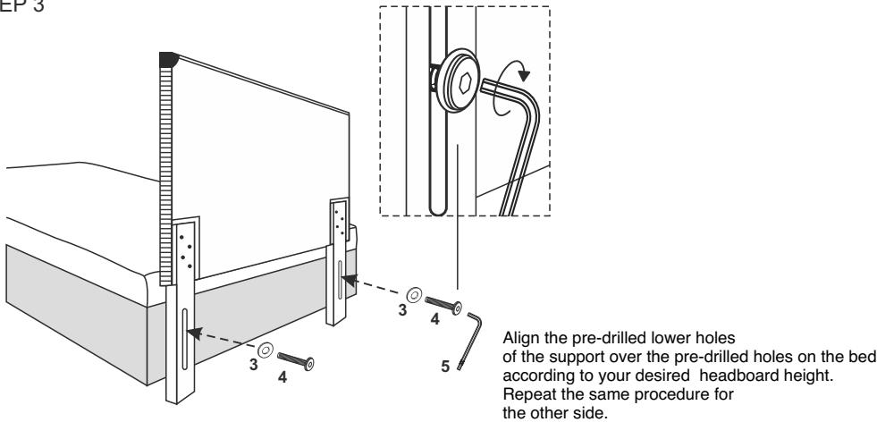
Align the pre-drilled lower holes of the support over the pre-drilled holes on the bed according to your desired headboard height.
