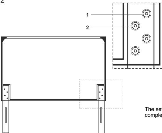
The set up of upper holes with stand upper holes is complete by securing all 8 bolts and 8 washers.
