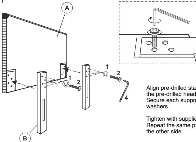
Align pre-drilled stand upper holes over the pre-drilled headboard holes
