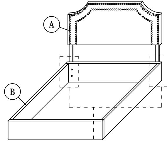
1. Line up the bed frame board's pre-drilled holes to match those of the headboard.
