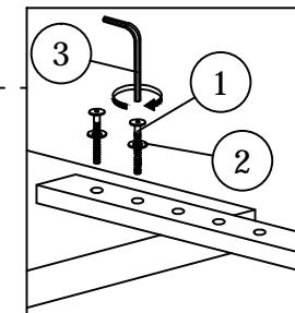
Secure each support stand by using 2x JCBB Bolt [1] and 2x M8 Flat Washer [2].
