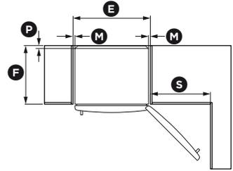
Flush with refrigerator chassis – full door rotation
