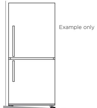
This foot lifts off the floor when top front is gently pushed back
