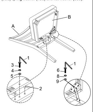
**STEP 2** Attach the legs (C) to the seat frame(B) using allen key (1) medium bolt (7) spring washer (8) and flat washer (9).
