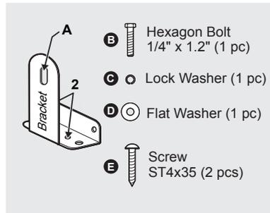
1. After you have chosen the installation location, place the bracket on the wood floor. Use Screw (E) (2 pcs) to secure bracket to floor using bracket holes (2).
