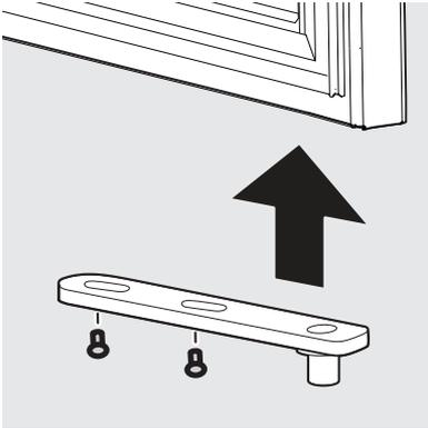
9. Place the metal washer and door on the bottom hinge pin and align with the top hinge pin (with the right upper corner of the gasket pulled back) and install the top hinge pin and metal washer. Place the hinge pin retainer in place on the door, push gasket in place.
