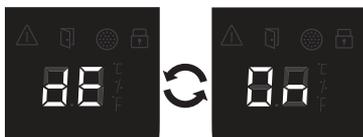
When deactivated, on Single, the display shows alternatively “dE” and “OF” for 5 seconds. Any alert turns off temporarily.
