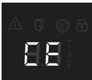
If the mode is set to Cellaring, the temperature display shows "CE" blinking. After 5 seconds without any interaction with the Mode button, the "CE" stops blinking and shows "CE" until the Cellaring mode is deactivated. When deactivated, the previous temperature is shown.
