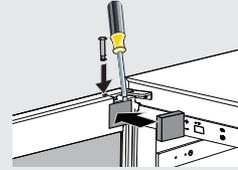
Hinge pin/hinge pin retainer
