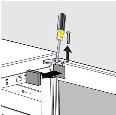
2. Lift the door from the bottom hinge pin and unscrew the bottom hinge from the unit, retain the metal washer from the hinge pin.
