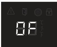
The default setting for Control Sounds is On. Press once to toggle the display between ‘OF’ and ‘On’. The ‘OF’ or ‘On’ will display for 2 seconds then the display switches back to the previous temperature setting.
