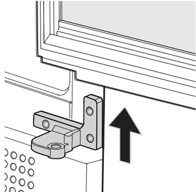
3. Unscrew the bottom hinge pin bracket from the bottom of the door. Place door on a padded surface to prevent damage.
