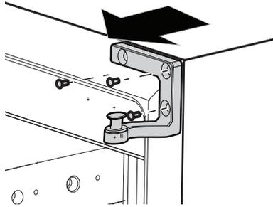
6. Carefully remove the left side top and bottom screw hole plugs and move to the opposite side of unit.
