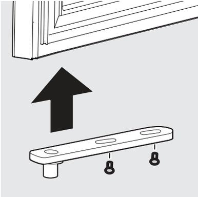
4. Remove the plastic cover located on the opposite side of the door and place it where the hinge pin bracket was located.
