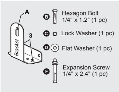
1. After you have chosen the installation location, use either hole (3) to secure the bracket into the concrete floor.
