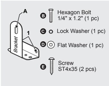
1. After you have chosen the installation location, place the bracket on the floor with (1) against the wall, use Screw (E) (2 pcs) to secure the bracket to the wall. Ensure at least one screw is secured into a stud.
