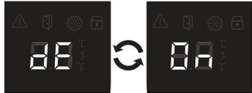
When deactivated, on Single, the display shows alternatively “dE” and “OF” for 5 seconds. On Dual, Lower & Upper temperature display shows and blinks “dE” and “OF” for 5 seconds. Any alert turns off temporarily.
