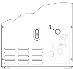
4. Locate water valve inlet and connect to valve.
