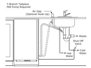
The maximum lift for the P60 drain pump is 10 feet. This must be done as close to the rear of the unit as possible.
