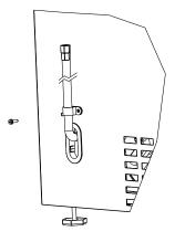
3. Thread water line through back panel hole (with bushing).
