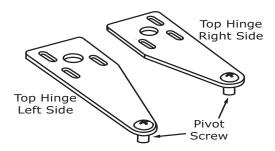
Remove pivot screw from hinge, flip hinge over, and install the pivot screw in the same hole from the opposite surface.
