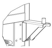
2. Remove corresponding screws on opposite side of cabinet. On some models there may be a nut behind one or both screws on either side.
