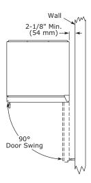
Units have a zero clearance for the door to open 90°, when installed adjacent to cabinets.
