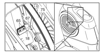
Next, rotate the Pulley (75) until a Magnet (67) is aligned with the Reed Switch (18). Slide the Reed Switch slightly toward or away from the Magnet. Then, retighten the M4 x 12mm Truss Head Screws (65).
