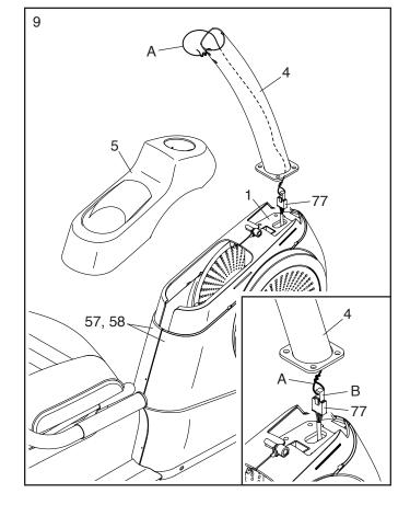
Do not pinch the Main Wire (77). Attach the Upright (4) to the Frame (1) with four M8 x 15mm Screws (24); start all four Screws, and then tighten them.
