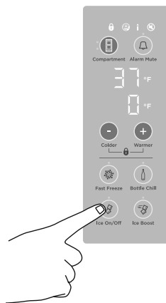
Turning ice maker on
