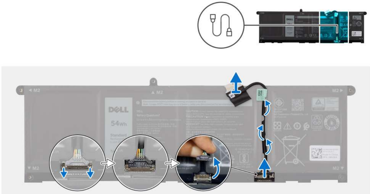
Figure 16. Removing the battery cable
