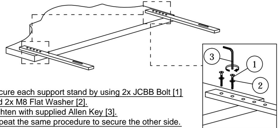
Secure each support stand by using 2x JCBB Bolt [1] and 2x M8 Flat Washer [2].
