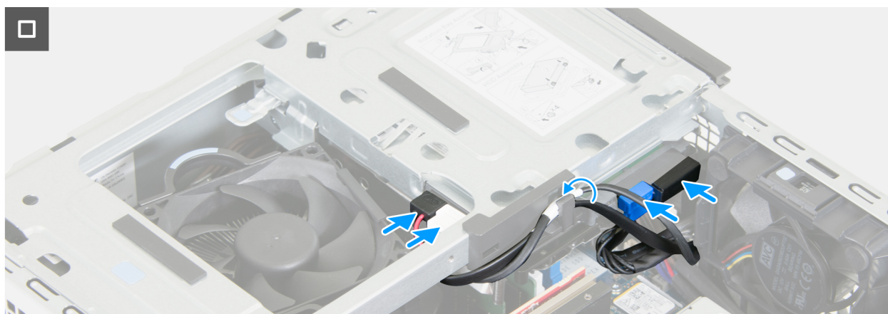
Figure 52. Installing the drive bay
