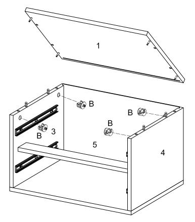
Place the top panel (1) to the side panels (3,4). Insert cam locks (B) into side panels (3,4) and tighten with a screwdriver.
