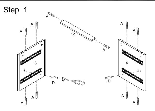
Insert dowels (A) into side panles (3)(4) and slat (12). Screw cam bolts (D) into side panels (3,4).
