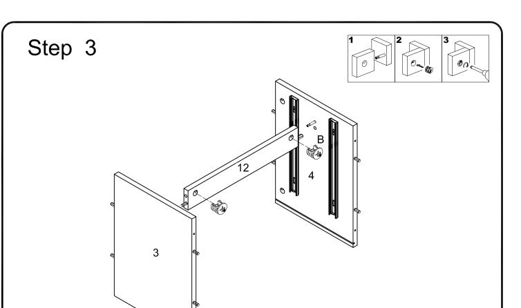
Attach side panels (3,4) to the slat (12). Insert cam locks (B) into slat (12) and tighten with a screwdriver.
