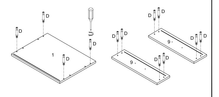
Screw cam bolts (D) into panels (1,9).
