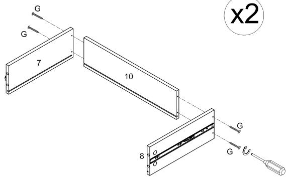
Use screw (G) to secure the drawer side panels (7,8) into drawer back panel (10).
