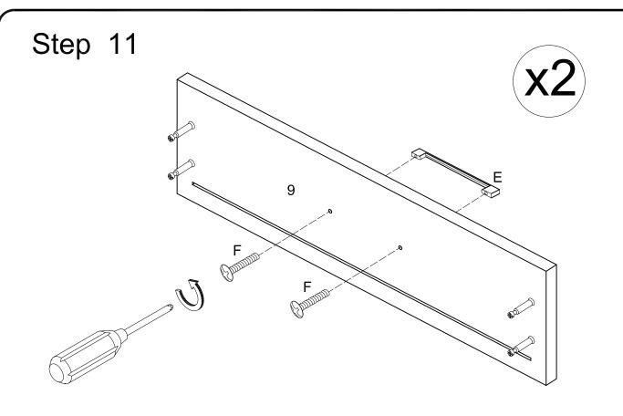
Secure handle (E) with bolts (F) into drawer front panel (9).
