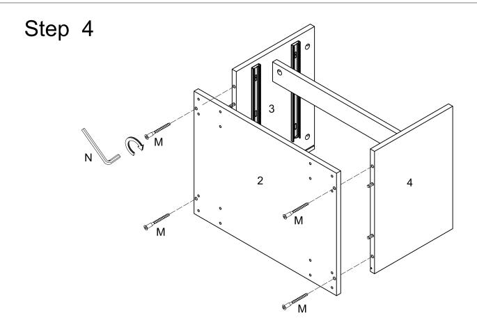
Use wrench (N), screw (M) to secure the bottom panel (2) to the side panels (3,4).
