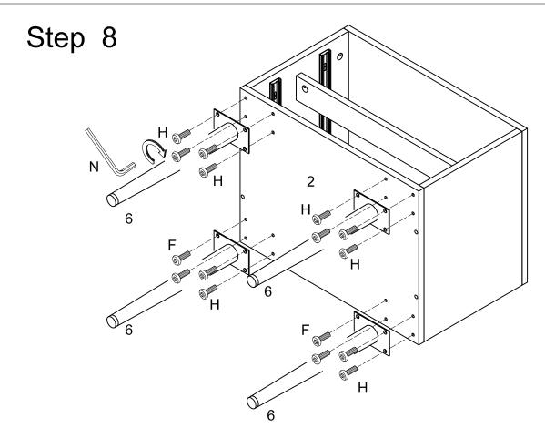
Use wrench (N), bolts (H) to secure legs (6) into bottom panel (2).
