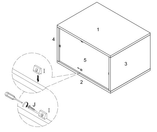
Secure the back panel (5) by using the plastic wedge (I) and screw (J).
