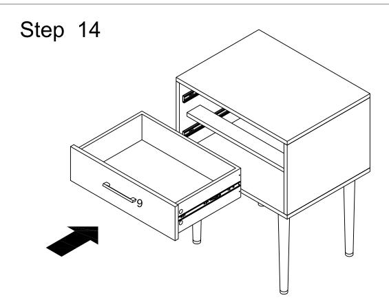
Carefully slide the drawer into the stand assembly. To remove the drawer, pull it out and press the small lever on the tray bracket, located inside the tray arm. Then carefully pull the two pieces apart.
