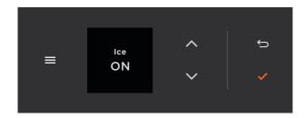
2. Press ✓ or ∧ to scroll to ICE, then press ✓ to turn the ice maker on or off.
