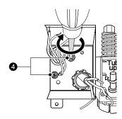
Pair the white, black, and green wires to the matching colored wires from the dishwasher. Then twist on the provided wire nuts **5** tightly to connect the corresponding wires.
