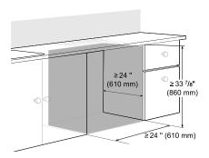
To allow for proper clearance of plumbing and electrical, use the template included with the literature to determine the clearance on the side of the cabinet where the cabinet meets the back wall. Using a 2 1/2" diameter hole saw, drill a hole in the target area as shown.
