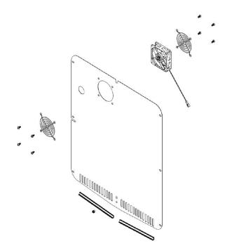
12. Remove and replace fan. Take special care to properly route fan wire.
