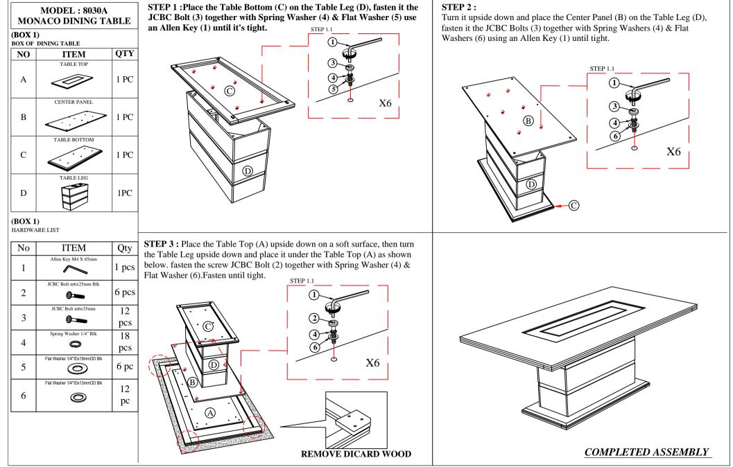
NOTE : MUST TIGHTEN SCREWS PERIODCALLY OR SCREWS WILL BECOME LOOSE.CHECK TIGHTNESS OF ALL SCREWS EVERY 6-8 WEEKS.
