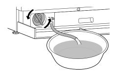
**5** Clean the pump filter and opening.
