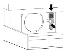
7 Insert the drain pump filter and twist it clockwise.
