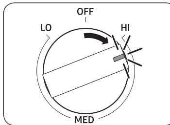
Press and turn the knob to a desired setting. The indicator turns on and confirms the selected setting.
