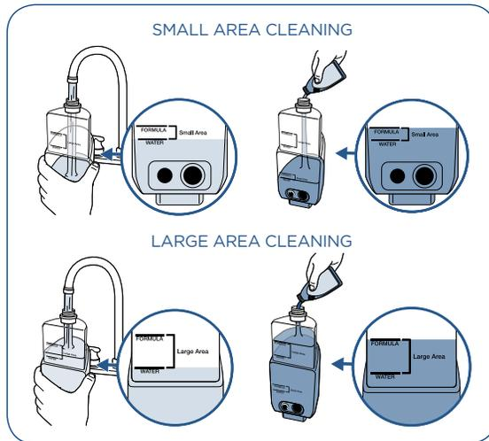
**2.** For small area cleaning (<350 sq ft), fill the clean water tank with warm tap water to the first water fill line. Then add formula to the first formula fill line.
