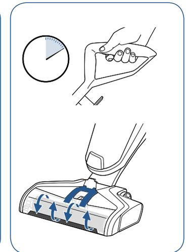
**5.** Each time you use the product, hold the solution trigger for 10 seconds to prime the system with cleaning solution before you begin cleaning. When you hold the trigger, LED lights will illuminate.
