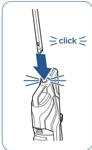
**1.** First, insert the handle at the top of the body of the machine until you hear a click.
