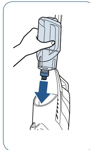
**3.** On the back of the machine, align clean water tank with the grooves and slide tank into place until you hear a click.
