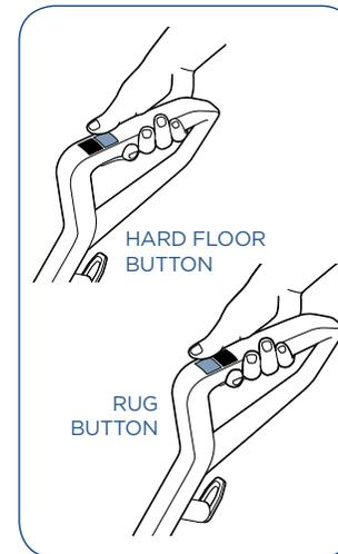
**4.** Turn machine on by selecting the type of floor you will be cleaning. For hard floors, choose the **HARD FLOOR** button and for area rugs push the **RUG** button.
