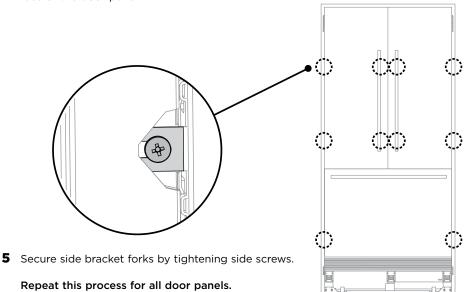
Note: for depth adjustment loosen side screws x4, adjust panels and then retighten once satisfied.
