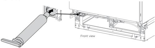
**2** Pull the freezer drawer out slightly and insert the filter cartridge and tool into the bottom left of the product. Firmly push the cartridge in until the filter head cannot be pushed any further.
