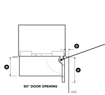
For  $90^{\circ}$  door swing a hinge limiting pin is supplied with your appliance. This pin fits in the boreholes of the top hinge (refer to  $\mathbf{Z}$ ).
