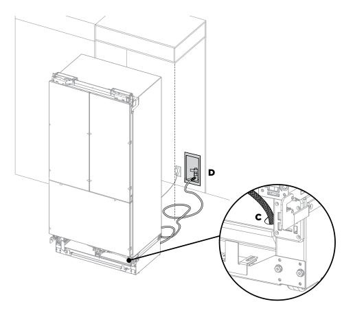
**6** At the back of the appliance, loosely coil the water hose (-2 - 3 times) and fasten the end of the hose to the cold water supply (refer to **D**).
