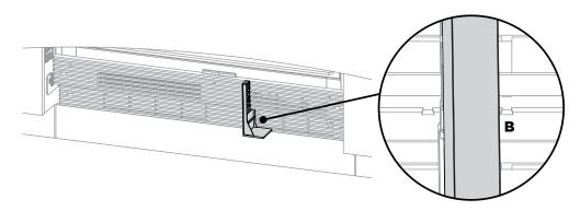
**2** Align the air flow divider underneath the grille tabs indicator and clip onto the vanes of the bottom grille (refer to **B**).
