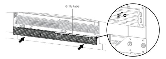
**3** With the grille tabs facing upwards, align the grille to the bottom of the plinth where the screw holes are located and secure with screws x3 (#8 x % pan head screws) (refer to **C**).
