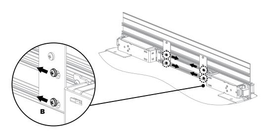
**5** Slide the screws located on the appliance sideways towards the narrow side of the key holes on the joining bracket, and tighten screws to lock top trim in position (refer to **B**).
