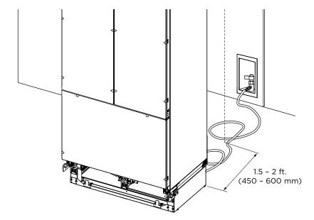
**2** At the front of the appliance, fasten the adaptor onto one end of the braided water hose.
