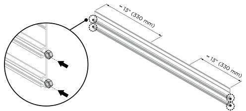
2 On the right side of the top trim, insert M5 nuts x2 onto the top and bottom slide. Slide nuts towards the center of the trim, ~ 13" (330 mm).
