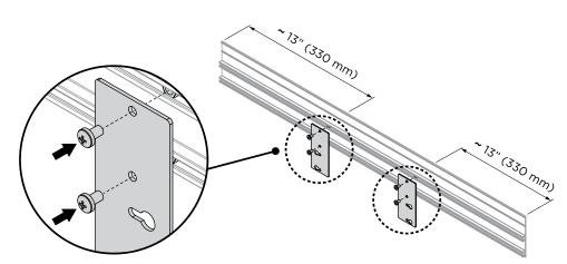
**3** Position joining brackets over the M5 nuts. Thread screws x2 (M5 x 8 pan head Phillips screws) through bracket hole and secure.
