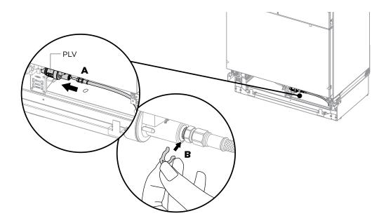
**4** Secure connection by attaching the locking key in between the PLV and tube end of the adaptor (refer to **B**).
