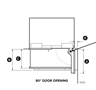
For  $90^{\circ}$  door swing a hinge limiting pin is supplied with your appliance. This pin fits in the boreholes of the top hinge (refer to  $\mathbf{Z}$ ).
