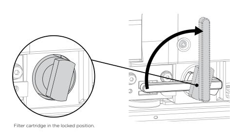
**3** Turn 90° clockwise to tighten. Remove filter cartridge tool and close freezer drawer.
