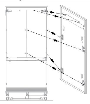
**3** All door panels have full axis adjustment to ensure they are flush with adjacent walls. To adjust the height of each panel turn clockwise to raise stud or counter-clockwise to lower stud (refer to **A**).
