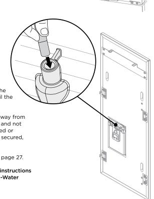
**6** Firmly push the water tube into the spigot behind the door panel until the marked line is not visible.
