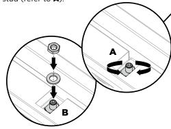
**4** Once satisfied with all door panels, secure M8 studs with M8 washer and M8 nut (refer to **B**). The top of the stud must remain below the top face of the door panel.
