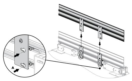
4 At the top of the appliance, place the assembled top trim behind the existing appliance trim. Bring the top trim forward and insert screw heads through the key holes of the joining brackets (refer to A).
