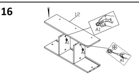
Align shelf mid side board (#12) to shelf boards (#22), then secure by using cam locks (#A1).
