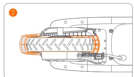
First clean up the foreign objects, and then wipe clean with a soft wet cloth. Lubricate both sides of the bearing with lubricating oil or machine oil. If the problem still exists, please contact customer service.
