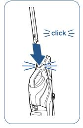
1. First, insert the handle at the top of the body of the machine until you hear a click.
