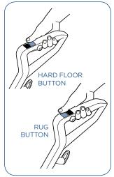
4. Turn machine on by selecting the type of floor you will be cleaning. For hard floors, choose the HARD FLOOR button and for area rugs push the **RUG** button.
