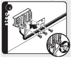
Attach the white (neutral) and black (line) lead to terminals. Attach ground wire to the center terminal.
