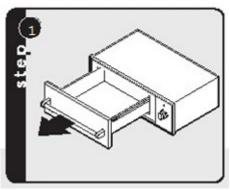
Pull out drawer assembly until fully extended
