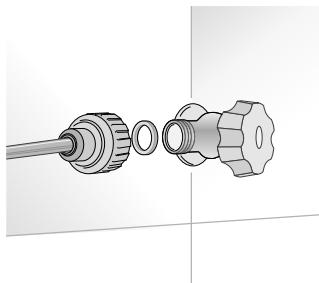
The models provided with Ice Maker require a connection to the domestic water supply system. This can be executed through the 1/4" water line (copper or polyethylene) to the house water supply.
