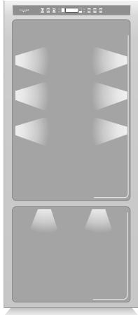
To provide optimum interior lighting, LED strips illuminate the refrigerator compartment from the top and sets of LED lights directly illuminate different areas of the refrigerator compartment, of the Crisper-Fresco drawers and the freezer drawer.
