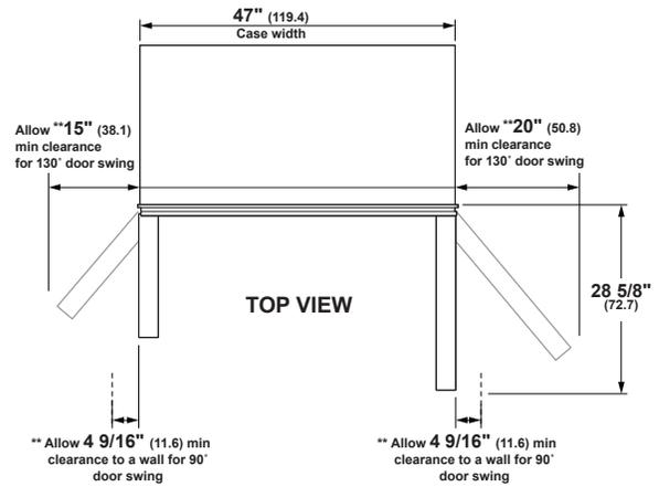
\*\* These refrigerators are equipped with a 3-position door stop. The factory-set 115° door swing can be adjusted to 90° if clearances to adjacent cabinets or walls is restricted. Allow full 130° door swings for pan removal. If the 90° door stop position is used, pan access is maintained, but pan removal is restricted. Dimensions based on custom handle height of 2 9/16" (6.5).
