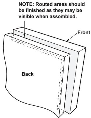
**CORNER VIEW SHOWING "PICTURE FRAME" ROUTING**
