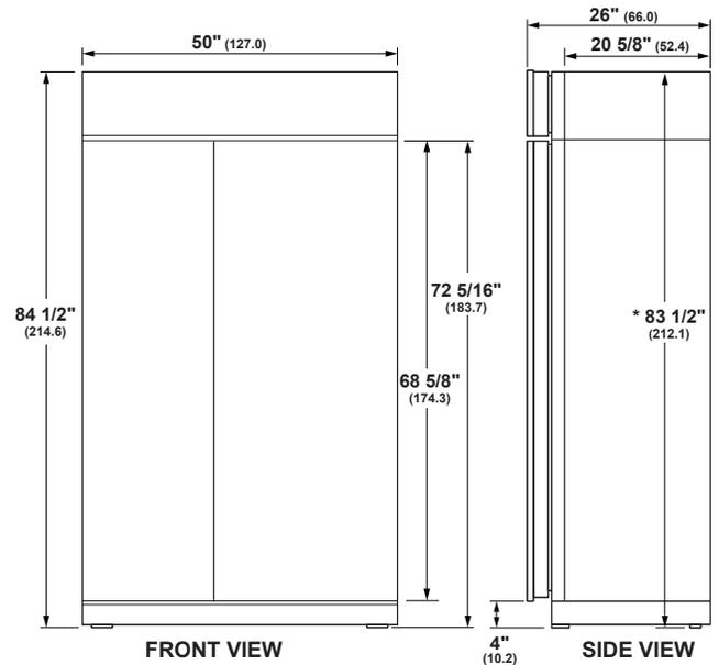
Use leveling legs and wheels for maximum 1" height adjustment from shipping height. Nominal installation height is 84".
