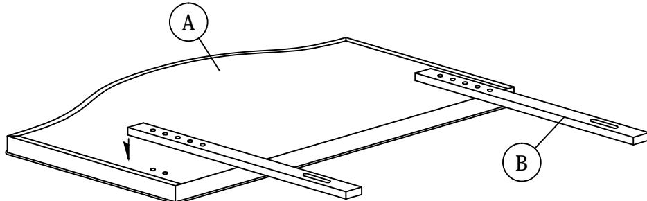
Align pre-drilled support stand holes over the pre-drilled headboard holes according to your desired headboard height
