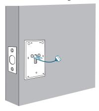
3. Attach the side with the silicone pad to the door, and secure the mounting plate with screws.
