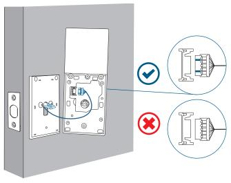
5. Insert the T-shaped tailpiece of the exterior keypad into the T-shaped tailpiece receiver of the interior assembly. Make sure the wire is tucked into the cavity on the back of the interior assembly.
