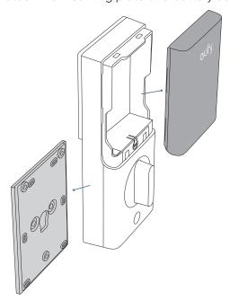
2. Run the cables through the slot on the mounting plate. Make sure the silicone pad is against the door.
