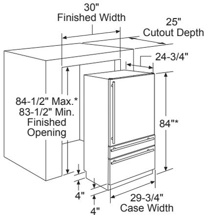
\* 84" High installation. The refrigerator can be adjusted to fit into a cutout that is 83-1/2" min. to 84-1/2" max with the appropriate door kit. Use leveling legs and wheels for a maximum 1" height adjustment.
