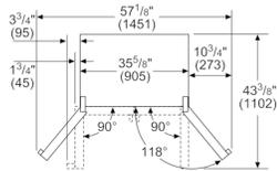
Drawers can be pulled out with door open to 90°. Drawers can be taken out with door completely opened.
