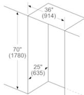
Leave 1/2" (12.7) gap at the top and 1" (25.4) behind the refrigerator for proper ventilation.
