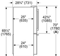
A: Add 1/2" (12.7) with front leveling feet fully extended
