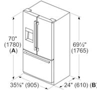
A: Add 1/2" (12.7) with front leveling feet fully extended
