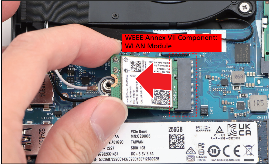
Figure 1-14. Removing the WLAN Module
