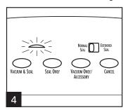
Wait until light turns green before letting go of lid and removing bag. Allow unit to cool 20 seconds between each use.
