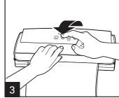
Close and hold lid; then press Seal Only button. Continue holding lid closed during entire sealing process.
