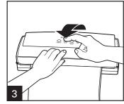
Close and hold lid; then press Seal Only button. Continue holding lid closed during entire sealing process.
