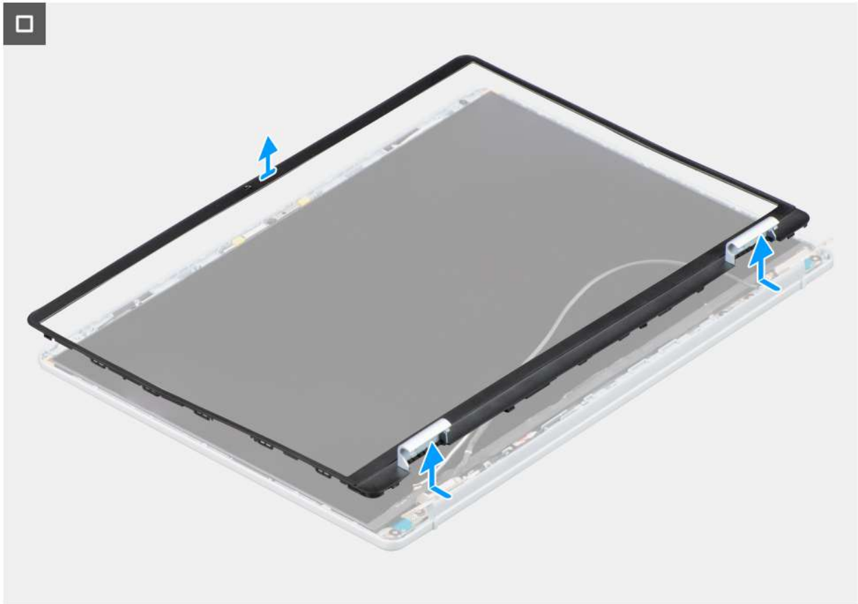
Figure 58. Removing the display bezel
