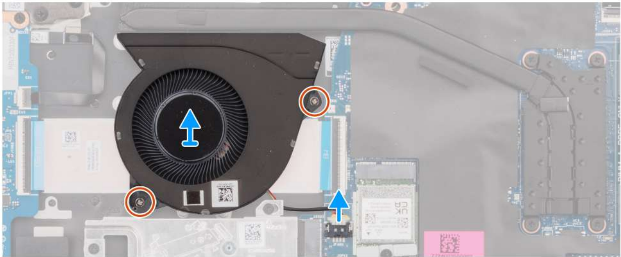
Figure 38. Removing the fan
