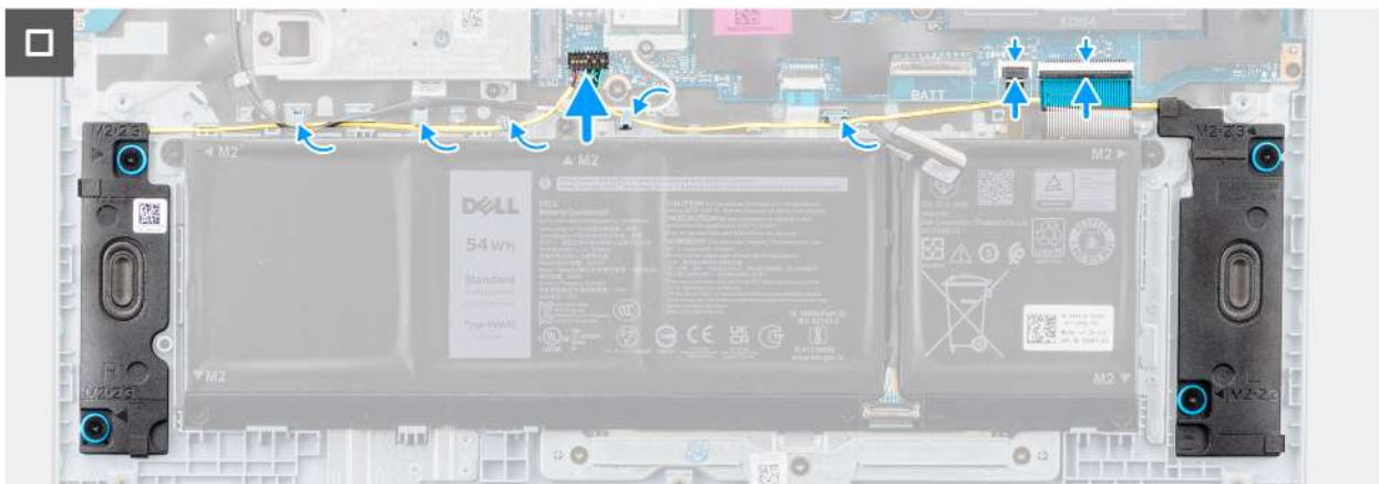
Figure 35. Installing the speakers
