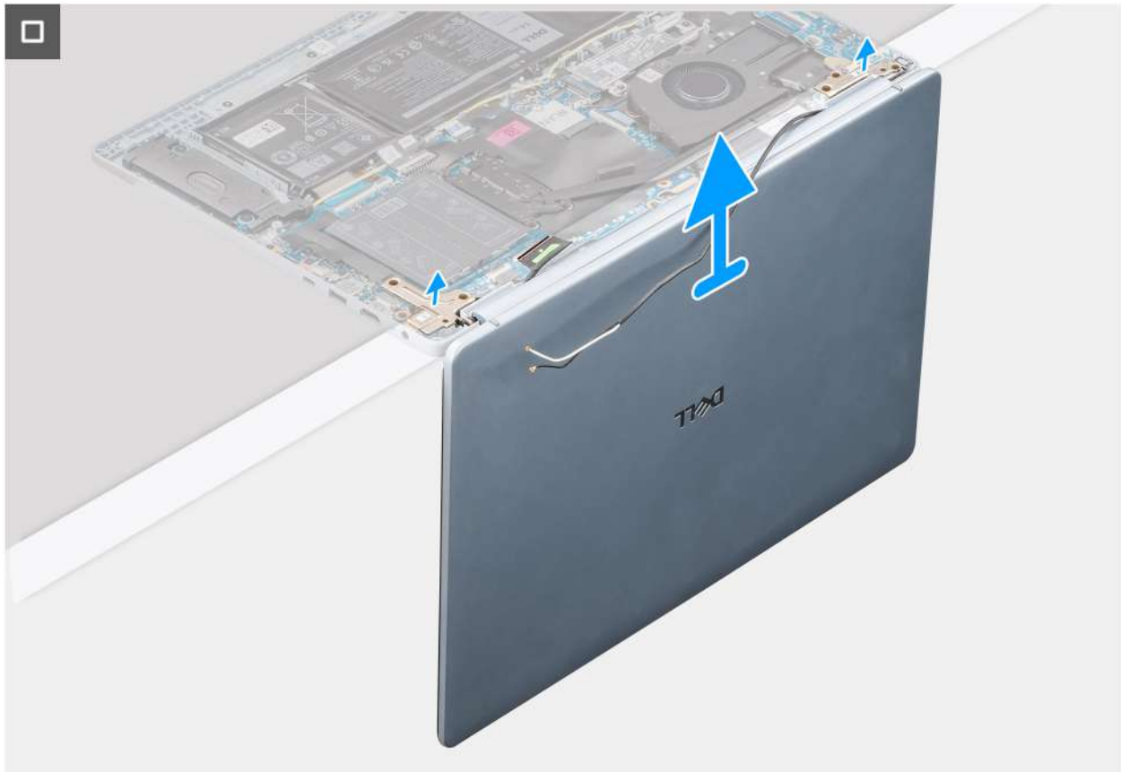
Figure 51. Removing the display assembly
