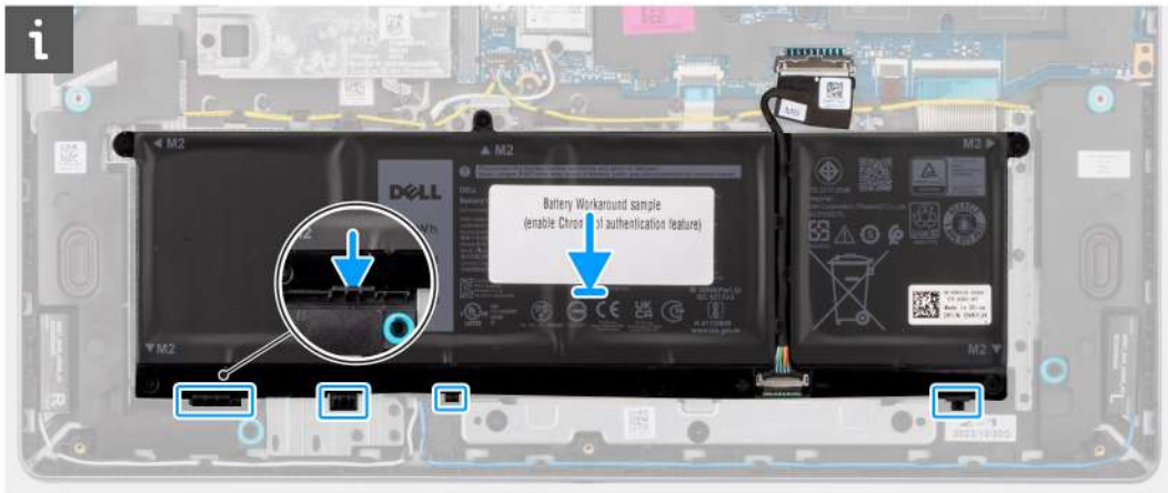
Figure 18. Installing the battery - Insert the tabs into hooks
