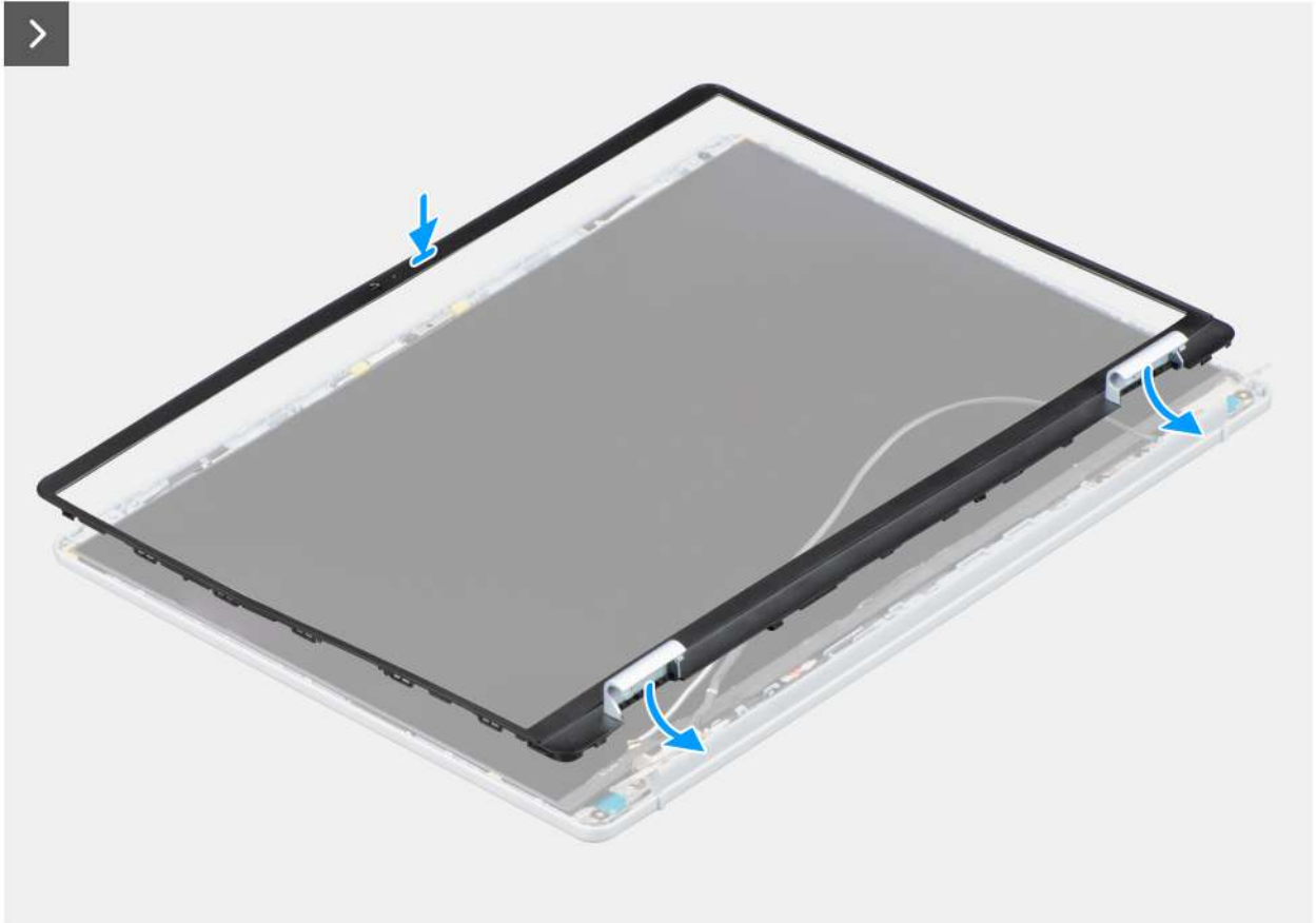
Figure 59. Installing the display bezel
