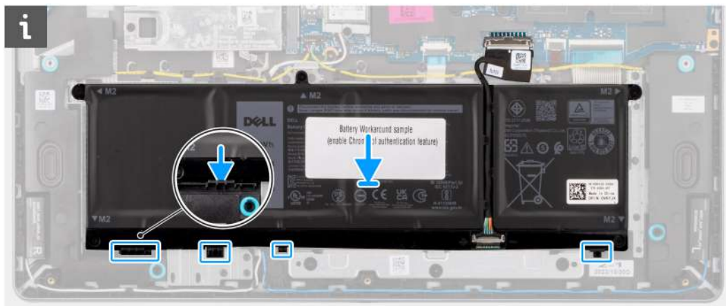
Figure 21. Installing the battery - Insert the tabs into hooks
