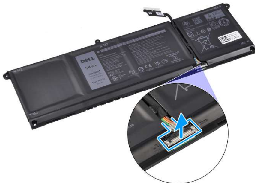
Figure 24. Disconnecting the battery cable
