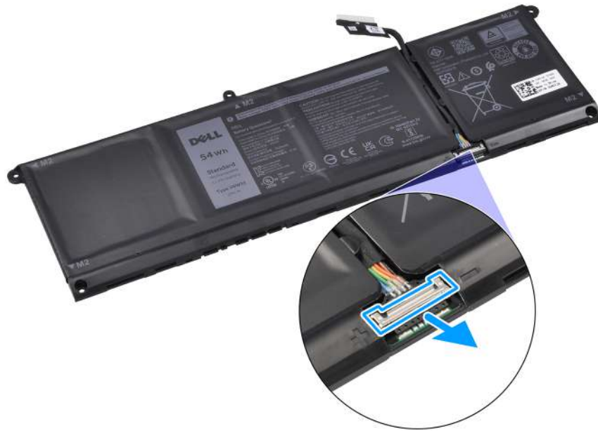
Figure 23. Releasing the battery cable connector
