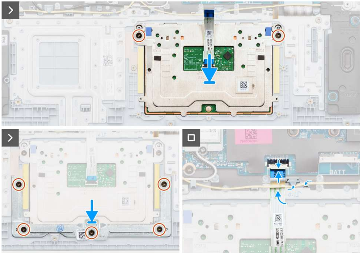
Figure 45. Installing the touchpad
