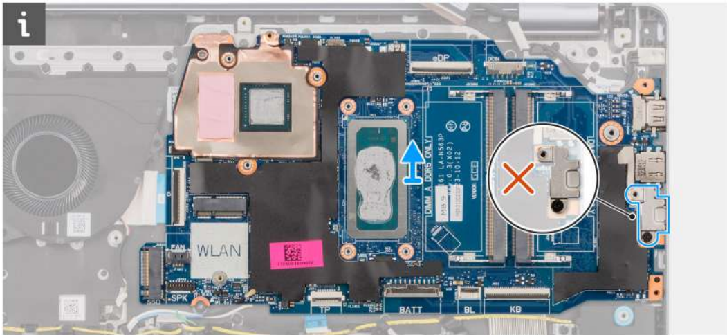
Figure 83. System board - USB Type-C bracket
