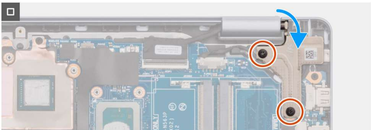
Figure 87. Installing the system board
