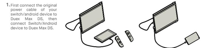
1. First connect the original power cable of your switch/android device to Duex Max DS, then connect Switch/Android device to Duex Max DS.
