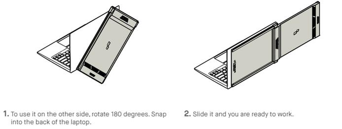
1. To use it on the other side, rotate 180 degrees. Snap into the back of the laptop.
