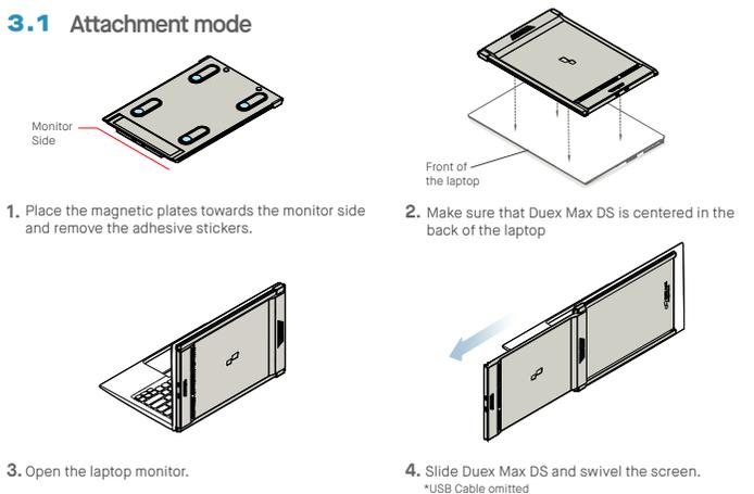
1. Place the magnetic plates towards the monitor side and remove the adhesive stickers.
