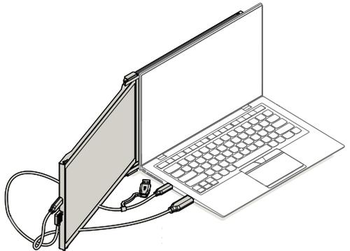
Using USB-C to C cable with HDMI cable
