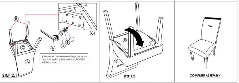
NOTE: MUST TIGHTEN SCREWS PERIODCALLY WITH USE SCREW WILL BECOME LOOSE CHECK TIGHTNESS OF ALL SCREW EVERY 6-8 WEEKS.
