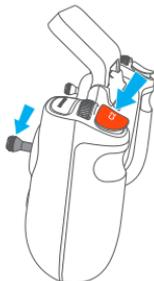
When the control stick mode is Mode 1 (right hand throttle), press the C2 button and simultaneously pull down the right control stick for 2s to unlock the motors. Release the control stick first to take off; otherwise, release the C2 button first to stop the propellers from spinning.
