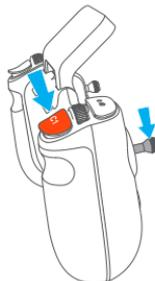
When the control stick mode is Mode 2 (left hand throttle), press the C1 button and simultaneously pull down the left control stick for 2s to unlock the motors. Release the control stick first to take off; otherwise, release the C1 button first to stop the propellers from spinning.
