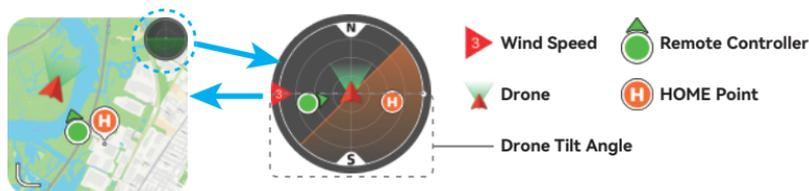
The attitude indicator displays information of drone direction, tilt angle, remote controller direction, HOME point and more.
