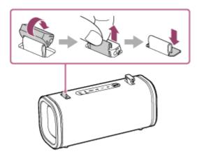
**3.** Rotate the storage cap on the right side counterclockwise as shown in the illustration. While pinching and lifting the attachment loop with your fingers, push the storage cap down.
