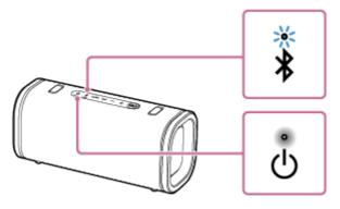
When the speaker has no pairing information, for example when you use the BLUETOOTH function for the first time after purchase, the  $\mbox{\ensuremath{\uptle}{R}}$  (BLUETOOTH) indicator on the speaker keeps double flashing in blue.
