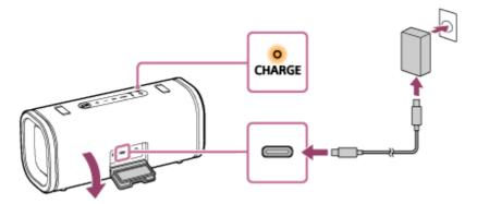
The CHARGE indicator on the speaker lights up in orange while charging is in progress and turns off when charging is complete.
