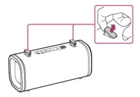
**2.** Rotate the storage cap on the left side clockwise as shown in the illustration. While pinching and lifting the attachment loop with your fingers, push the storage cap down.
