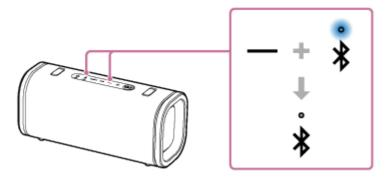
When you press and hold the – (volume) button and the 3 (BLUETOOTH) button simultaneously for about 5 seconds once again, the 3 (BLUETOOTH) indicator flashes and the BLUETOOTH function turns on.
