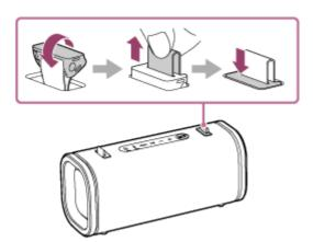
**4.** Pass the hooks of the shoulder strap through the left and right attachment loops.
