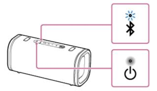
When the speaker has no pairing information, for example when you use the BLUETOOTH function for the first time after purchase, the **\$**(BLUETOOTH) indicator on the speaker keeps double flashing in blue.
