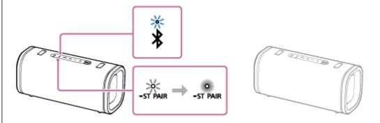
On the other speaker, press and hold the ★(BLUETOOTH)/ ST PAIR (Stereo Pair) button for about 2 seconds.
