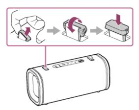
**3.** Hook your finger on the tab of the storage cap on the right side and lift it up. Rotate the storage cap clockwise as shown in the illustration and push it down.
