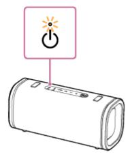
If an abnormality is detected, disconnect the USB cable, wait for a while, and then restart the speaker (by pressing and holding the () (power) button on the speaker for about 10 seconds). If the problem persists, contact Sony support contact or your nearest Sony dealer.
