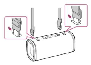
2. Hook your finger on the tab of the storage cap on the left side and lift it up. Rotate the storage cap counterclockwise as shown in the illustration and push it down.
