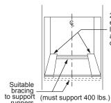
equivalent runners level with bottom of cutout and flush with sides of cutout or solid bottom floor.
