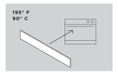
Reactivate the carbon filter. Place in oven for 60 min at 195°F (90°C). Refit filter to recirculation kit and replace grille.
