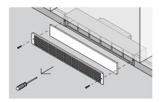
Remove the stainless grille by removing screws with crosshead screwdriver.
