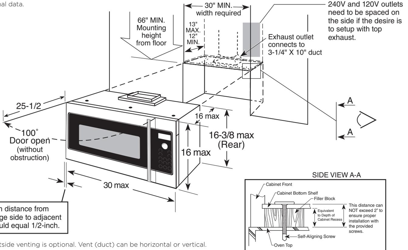
Minimum distance from door hinge side to adjacent wall should equal 1/2-inch.
