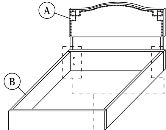
1. Line up the bed frame board's pre-drilled holes to match those of the headboard.
