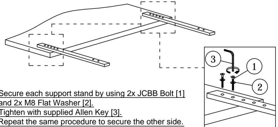
Secure each support stand by using 2x JCBB Bolt [1] and 2x M8 Flat Washer [2]. Tighten with supplied Allen Key [3]. Repeat the same procedure to secure the other side.
