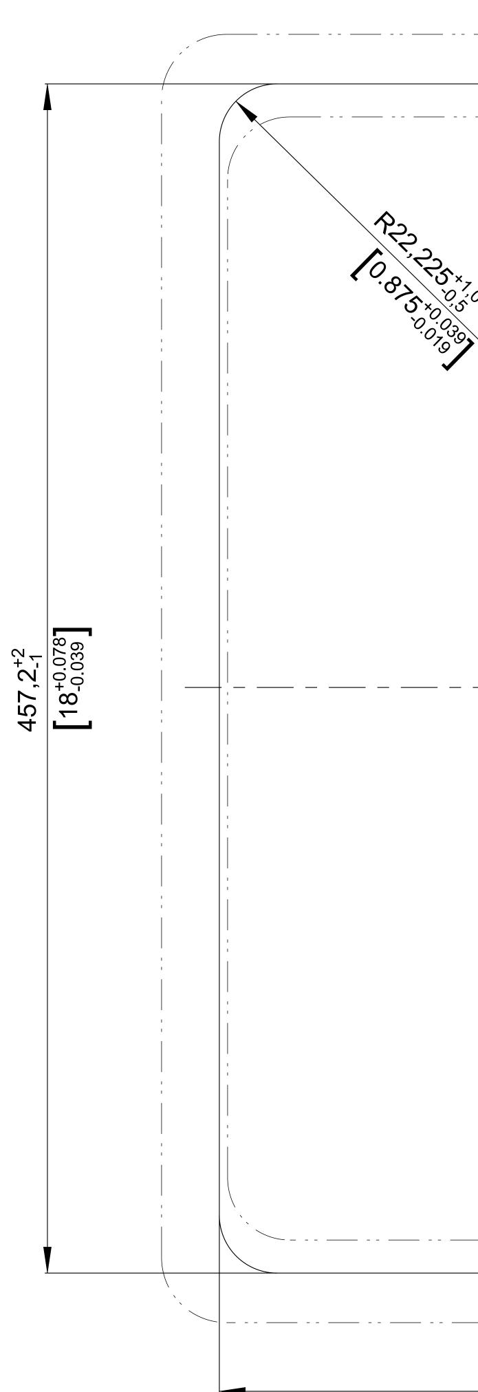
For sinks with undermount installation the shown dimensions and tolerances mu
