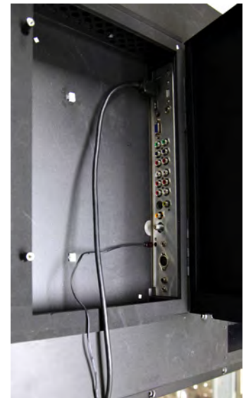
Place IR Emitter Cable over the bottom of the cable door.
