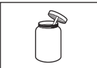
Pipe-joint compound resistant to propane gas
