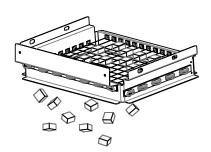
The bin level sensor is located in the ice bin, it senses when the ice supply is low or full and starts or stops the ice making process accordingly.
