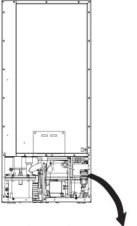
To disconnect the water outlet line: Push up on the white collar and pull the plastic water line from the bottom of the water valve.
