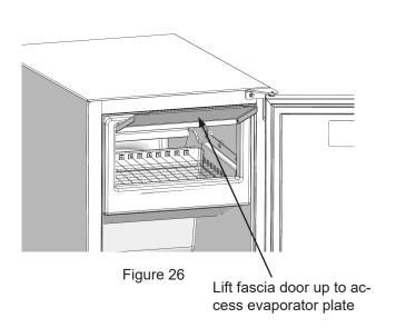
Remove ice from bin. Pull plug from the reservoir. Once reservoir is empty, replace plug. Hold the button for 10 seconds to show "CL" on the display. Lift Fascia door to access evaporator plate. Lift or remove splash shield to expose evaporator plate. Using 1-3 ounces of cleaner, pour cleaning solution slowly on evaporator plate so it flows down into the fresh water reservoir.
