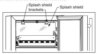
Replace the splash shield if removed.
