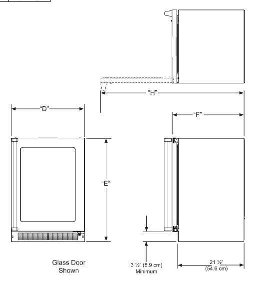
Minimum rough-in opening is required to be larger than the adjusted height of the cabinet.
