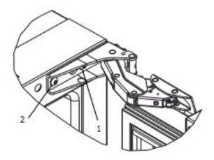
Once door is removed, using a Philips Screwdriver, remove screws from magnet actuator located on inside and bottom of door (On integrated models, magnet actuator will be located on bottom of door.
