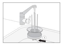
■ Rinse the milk pipework in the lid under running water.
