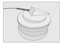
■ Use the cleaning brush to clean the milk pipework in the lid as well.
