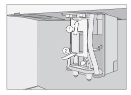
■ Push the catch upwards ①, grasp the dispensing unit by the handle and pull it out towards the front ②.
