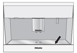
Replace the cover onto the drip tray. Make sure that the front of the cover is flush with the drip tray.
