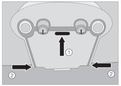
■ To remove, press and hold the sensor cover between the dispenser nozzles ①. Then press the main dispenser in from the sides at the back ②.
