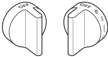
Electric igniters automatically light the surface burners when control knobs are turned to
